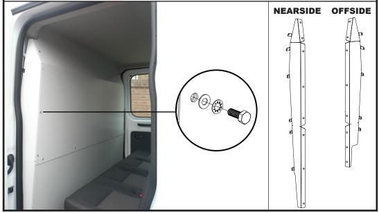
Once happy with the position of the bulkhead carefully drill 3.2mm through the fixing tabs and into the vehicles 'B' pillar. Secure to the pillar using No8x1/2" self-tap screws (FX4090) (11 positions).
