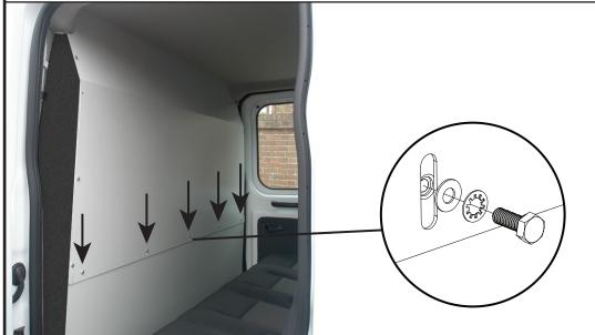
Secure the sides to the bulkhead using M6x16 hex bolts (FX4012), M6 shakeproof washers (FX4010) and M6 washers (FX4017) (8 position each side). Once the sides are in position lift the top bulkhead upwards to the top of the roof and tighten all fixings.
