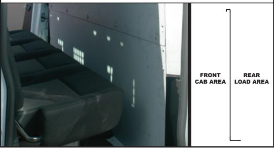
Lift the top bulkhead into the vehicle and **loosely** secure to the bottom bulkhead in 5 positions using M6x16 hex bolts (FX4012), M6 shakeproof washers (FX4010) and M6 washers (FX4017).
