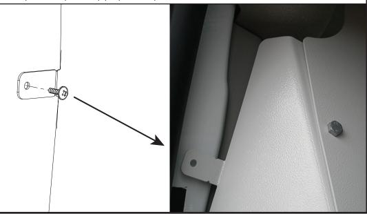
Carefully drill 3.2mm through the 5 positions along the bottom flange of the bottom bulkhead and secure to the vehicle using No8x1/2" self tap screws (FX4090).
